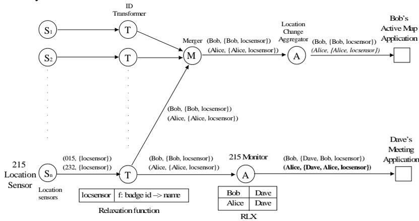
Notice that events pass through the stateless Merge operator with unchanged ACLs. The Location-Change Aggregator takes care to use a separate state object  $s_p$  for each principal  $p$ , so that  $ACC_{i_s p} = \{p\}$  and those location events can pass through with unchanged ACLs. Although the aggregator publishes events about Alice, tagged with ACL  $\{Alice\}$ , Solar does not deliver those events to the Active Map application run by Bob (see Section 5.2).
