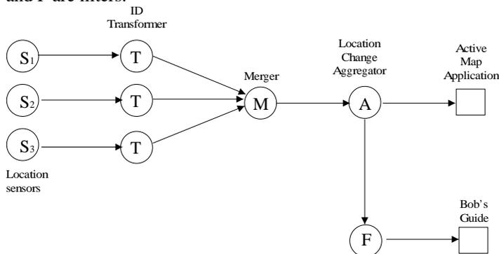
*Architecture.* The Solar system is distributed across many hosts, although the only abstraction presented to operators and applications is the operator graph [3,4]. Applications run outside the Solar system, on any platform, using a small Solar library that allows them request subscriptions and to receive events over standard network protocols.
