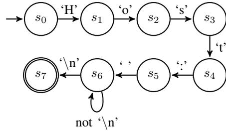
Fig. 1. A simple DFA that recognizes the HTTP “Host” header. Note that if a transition does not exist for a given input character from a given state, the entire input is rejected. State  $s_0$  is the start state and state  $s_7$  is the accepting state.
