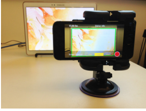
Figure 9: Experimental setup with Samsung Tab S (left) as the transmitter and iPhone 5s as the receiver (right).
