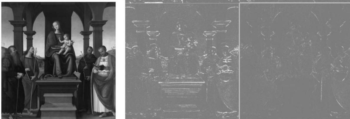
**Fig. 4.** The absolute values of the subband coefficients at three scales and three orientations (the residual low-pass subband is shown in the upper left corner) (Right) for the Perugino painting (Left).
