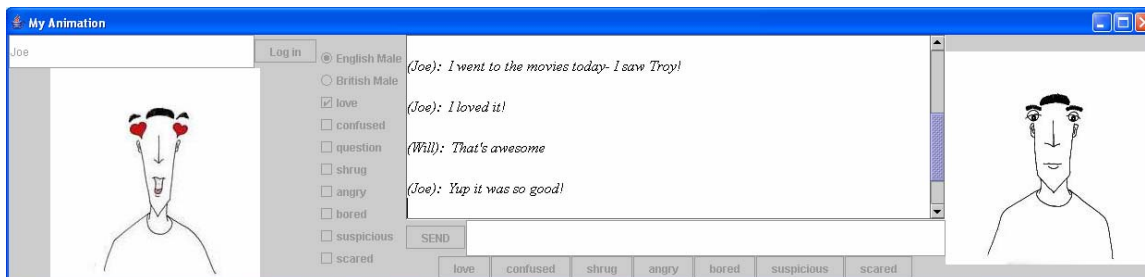
Figure 11. Chat messages are displayed in the center text box. Text input is transmitted to X-Speech by typing a message and pressing the “send” button. The left avatar in the GUI is the displays the sender’s animations, and the right avatar displays the received messages.
