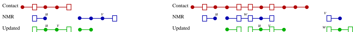
Fig. 3. Reuse-based growing and aligning. Contact graph and NMR residues in the same column are matched. There are two amino acid types (empty squares and filled circles), which must match. (left) Growing from a matched fragment ending in u to an unmatched fragment with v in the middle leaves behind the prefix of the unmatched fragment in order to append and match the suffix following u . (right) Growing from u to v requires a realignment of the joined fragment. The joined fragment displaces the suffix starting at w of another fragment.
