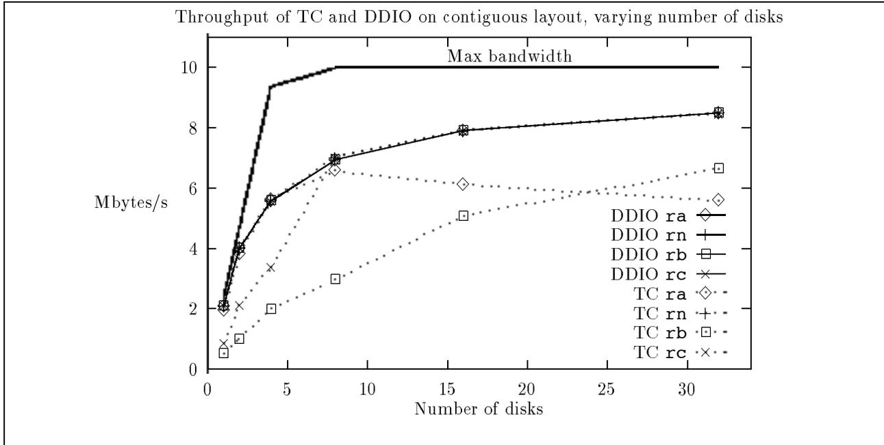
Figure 7: A comparison of the throughput of disk-directed I/O (DDIO) and traditional caching (TC), as the **number of disks varied**, for the ra, rn, rb, and rc patterns (ra throughput has been normalized by the number of CPs). All cases used the contiguous disk layout, and all used 8 KB records. The maximum bandwidth was determined either by the disks (1–4 disks) or by the (single) bus (8–32 disks).
