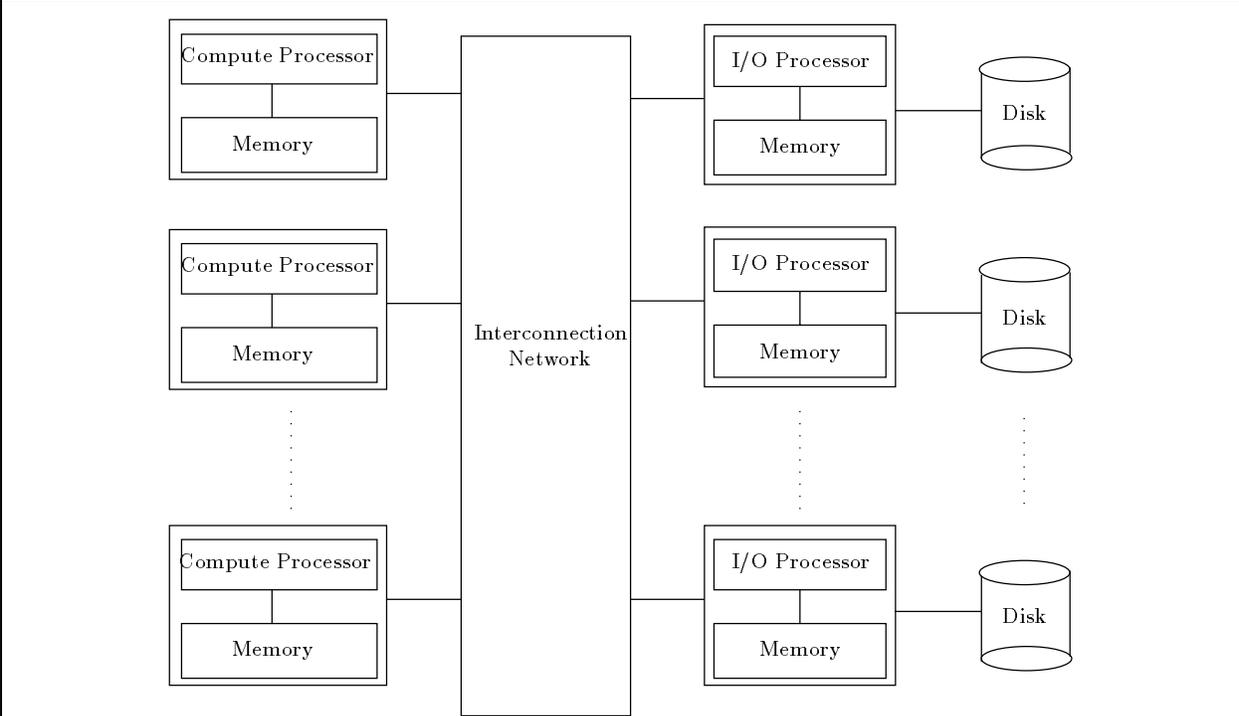
Figure 1: An architecture with two types of processor nodes: compute processors and I/O processors. The latter have attached disks and are dedicated to file-system service.
