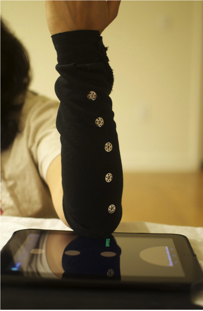
Fig. 2. Protective cover to minimize skin contact with the touchscreen
