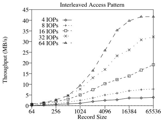
Figure 4: Throughput for write requests using the traditional Unix-like interface. There were 16 CPs in every case.
