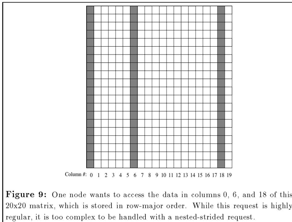
**Figure 9:** One node wants to access the data in columns 0, 6, and 18 of this 20x20 matrix, which is stored in row-major order. While this request is highly regular, it is too complex to be handled with a nested-strided request.
