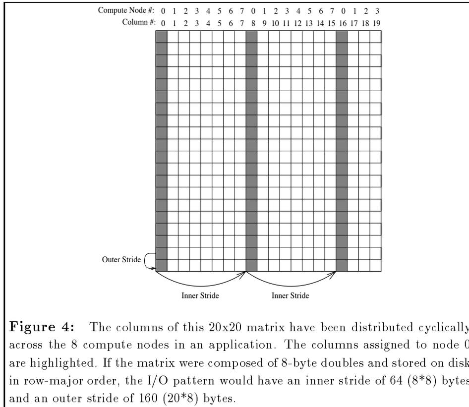
**Figure 4:** The columns of this 20x20 matrix have been distributed cyclically across the 8 compute nodes in an application. The columns assigned to node 0 are highlighted. If the matrix were composed of 8-byte doubles and stored on disk in row-major order, the I/O pattern would have an inner stride of 64 ( $8*8$ ) bytes and an outer stride of 160 ( $20*8$ ) bytes.
