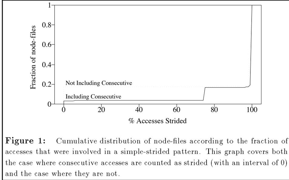
**Figure 1:** Cumulative distribution of node-files according to the fraction of accesses that were involved in a simple-strided pattern. This graph covers both the case where consecutive accesses are counted as strided (with an interval of 0) and the case where they are not.
