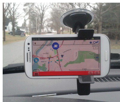
Figure 2: CarSafe, the first dual-camera sensing app, running on a Samsung Galaxy S3 mounted on the windshield of a car.
