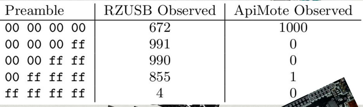
ApiMote's CC2420 RF chip was configured to default preamble length and SFD. Address and checksum verification was disabled.
