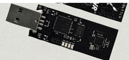
ApiMote's CC2420 RF chip was configured to default preamble length and SFD. Address and checksum verification was disabled.
