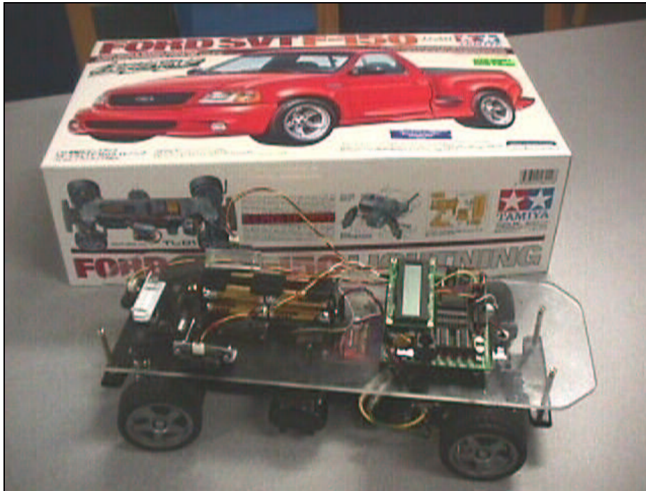
Figure 1. A Handy Robot with a Plexiglas electronic mounted on a Tamiya car base.
