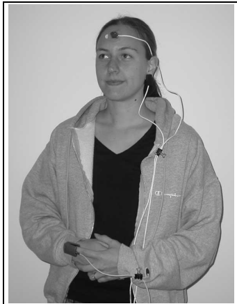
Figure 4. Placement of forehead, ear, and finger pulse oximeters on subject.
