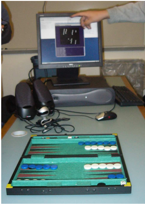
Figure 2. A camera hung from the ceiling is used to find a backgammon board and locate all the pieces for display on the computer screen. The program gives verbal descriptions of each detected move. Another team was responsible for reading the dice.
