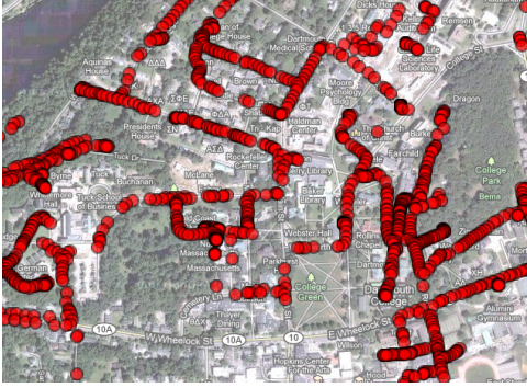
Figure 1. 802.15.4 packets captured on Dartmouth campus. Each circle represents a point where an 802.15.4 packet was logged.
