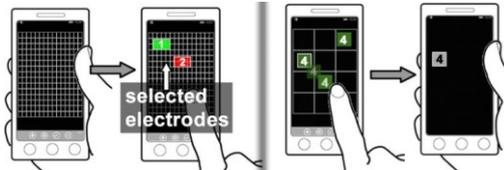
**Fig. 6.** Left: configuring a grid of  $15 \times 15$  electrodes; Right: duplicating a number key to configure a  $1$ -to- $m$  mapping.
