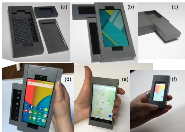
Figure 4. Hardware prototype: (a) 3D printed housings; (b) form factor showing medium and small pieces half slid out; (c) sliding mechanism; (d) large piece with medium piece half slid; (e) detached medium piece; (f) detached small piece.
