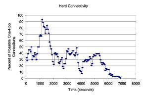
Figure 4: Connectivity among the herd, measured by the percentage of one-hop connections present relative to all pairs of cows. At the beginning of the experiment, the cows were tightly clustered, so that most collars could communicate directly with most others. In the field, the connectivity was less complete but still sufficient and fairly consistent.
