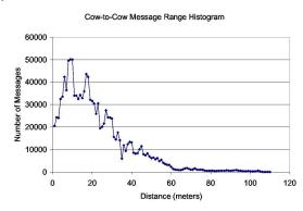
Figure 5: Distances over which messages were successfully sent. Range obtained from GPS positions of the cows sending and receiving messages.
