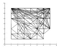
Figure 5: Measured communication graph of the experimental 7x7 grid network. Notice the absence of many point to point links we expect to be available (from example from (1,1) to (2,1)) and the presence of long links we do not expect to have, for example from (1,7) to (7,6).
