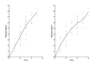
Figure 3: This figure shows the comparison between the measured real distance and the hops counted using our algorithm.
