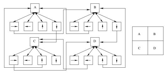
Fig. 8. Four zones are in a square network field. The power of a zone is evaluated in four directions, left, right, up, and down. A zone is represented as a zone vertex with four direction vertices. The power labels are omitted from this figure.
