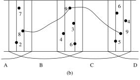
Fig. 7. Three zones, A, B, and C. SB, SC are the source areas of B and C, and TA, TB are the sink areas of A and B. AB and BC are overlap border areas. (b) shows how to connect the local path in zone B with the local path in zone C. The number next to each node is the number of paths passing through that node in the power evaluation procedure. The vertical stripes are the source and sink areas of the zones.
