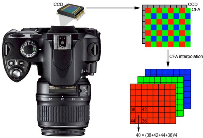
**Figure 1:** A color filter array (CFA) overlaid onto a CCD sensor. Each CCD element records a limited range of wavelengths, corresponding to either red (gray), green (light gray), or blue (dark gray). A full three channel RGB color image is created by interpolating the missing color pixels by, for example, averaging the recorded values.
