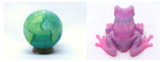
Figure 9: Examples of color shifting when filament is not properly lined up with the GCODE executed by the 3D printer. Globe and tree frog prints retain distinct colors though shifted throughout the print.
