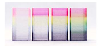
Figure 10: Sample of spiral vase mode prints using translucent PLA colored with black, cyan, yellow, and magenta inks with increasing perimeter counts. The number of perimeters in a print affects the strength of the perceived color. From left to right: single perimeter, two perimeters and three perimeters with no ink overlap, and three perimeters with 200 mm of ink region overlap between colors.
