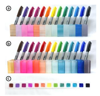
Figure 7: A comparison of color reproduction using 13 different colored permanent markers on 3D printed objects. (a) and (b) show the color results of ink applied to filament prior to 3D printing. (c) shows the color results of ink applied after 3D printing. Filaments used: (a) opaque white PLA, (b) translucent PLA, and (c) opaque white PLA.
