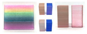
Figure 11: Color mixing samples producing varying effects; rainbow gradients made using CMYK color mixing (left), directionally dependent prints where certain colors appear stronger from different angles (middle), and mixing differences between opaque and translucent materials (right).
