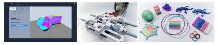
Figure 1: Automated filament inking is a novel system for producing multi-color 3D prints with an FFF printer. Shown is a collection of multi-color 3D prints created using our open-source low-cost inking device and web interface for producing custom filament profiles.
