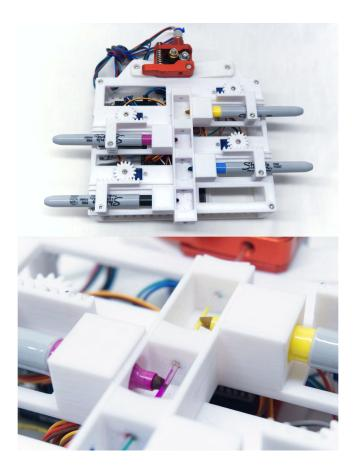
Figure 3: Our inking device loaded with cyan, magenta, yellow, and black permanent markers, inking translucent PLA filament.
