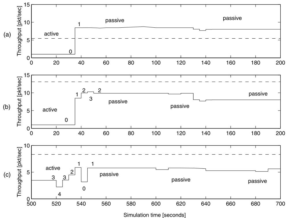
of passive periods is uniformly distributed between 150–800 seconds. The three graphs shown in Fig. 7 contrast the PCQoS operation of the test flow in different network conditions: In Fig. 7(a) only 10% of the flows in the network are gold flows, Fig. 7(b) same as (a) but with a higher target throughput, and Fig. 7(c) where 30% of the flows are gold flows.
