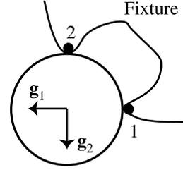
Figure 2: External wrenches that may cause contact to be broken at both fixels simultaneously.
