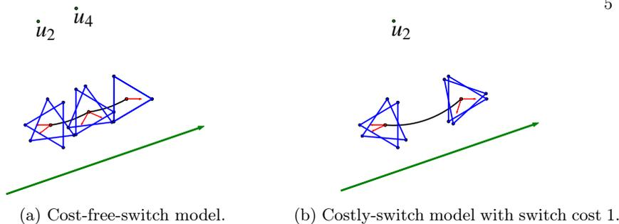
Fig. 2: Trajectories for an omni-directional vehicle starting at  $(-3, -1 \pi)$ . For the cost-free-switch model, the optimal trajectory takes 5 actions. For the costly-switch model, the (approximately) optimal trajectory takes 3 actions. Green lines are control lines.
