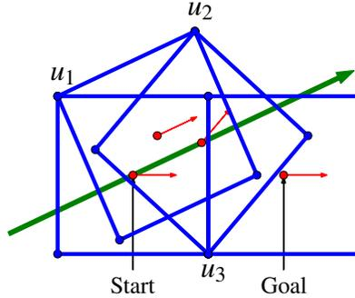
Fig. 1: An approximately optimal trajectory for a refrigerator robot starting at  $(-2, 0, 0)$ , with unit cost for switching between any pair of controls. The green line is the control line.
