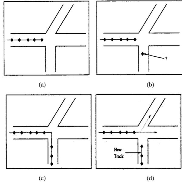
Fig. 3. An illustration of an ambiguous situation. (a) A track associated to a single vehicle exists. (b) A new observation from the same vehicle comes up. (c) Hypothesis 1 (right): The track is enlarged with the new observation. (d) Hypothesis 2 (wrong): A new track is created. Two vehicles are now assumed to be present in the scenario.
