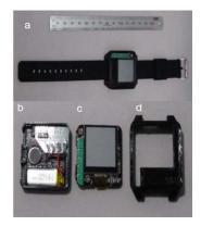
Fig. 1 (a) Fully assembled Amulet device; (b) internal Amulet peripherals; (c) screen; (d) case
