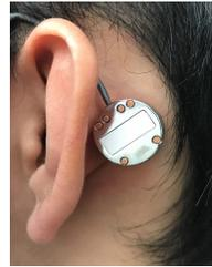
Figure 1: Contact microphone
