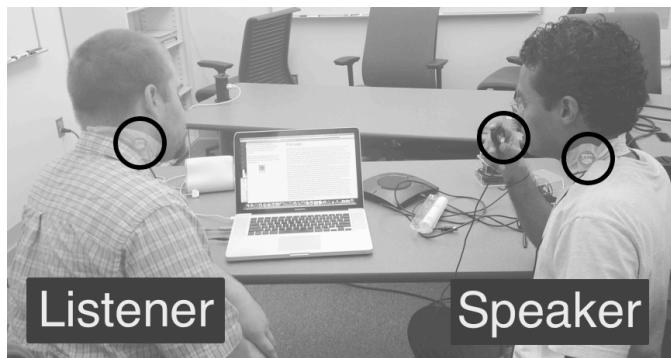
Figure 4: The sample collection setup. The microphone locations are indicated by circles.
