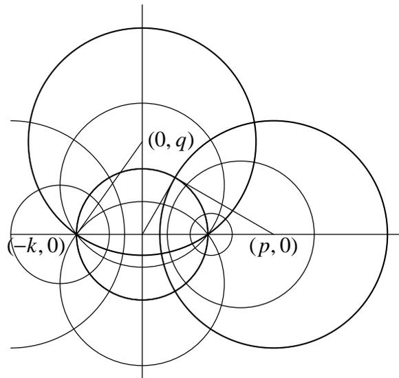
Figure 5. Representative members of two orthogonal systems of coaxial circles. Meridians are centered on the  $y$  axis and parallels on the  $x$  axis. Poles are at  $(\pm k, 0)$ . Meridians intersect parallels at right angles. Thick circles are a typical parallel centered at  $(p, 0)$  with squared radius  $p^2 - k^2$ , a typical meridian centered at  $(0, q)$  with squared radius  $q^2 + k^2$ , and the smallest meridian circle (radius  $k$ ).
