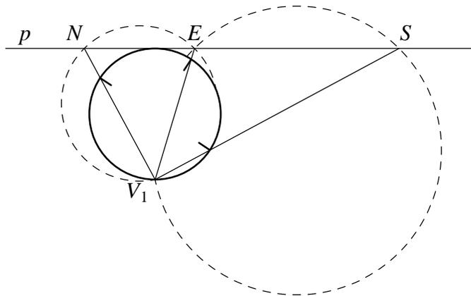
Figure 6. Back projection onto a standard sphere from an arbitrary coaxal system in plane  $p$  with poles  $N$  and  $S$ . A standard sphere, with tick marks at the poles and equator, is placed with a meridian tangent to the unique straight meridian in  $p$ . In  $p$ , the equator meets the straight meridian at  $E$ . The dashed circles are the loci of viewpoints from which  $NE$  and  $ES$  subtend  $\pi/4$ ;  $V_1$  is the unique viewpoint that achieves both.
