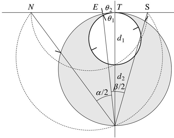
Figure 8. A standard sphere and a droopy sphere with a common point of tangency,  $T$ .  $\theta_1$  and  $\theta_2$  are azimuths of the equator measured at the center of the spheres relative to the point of tangency.
