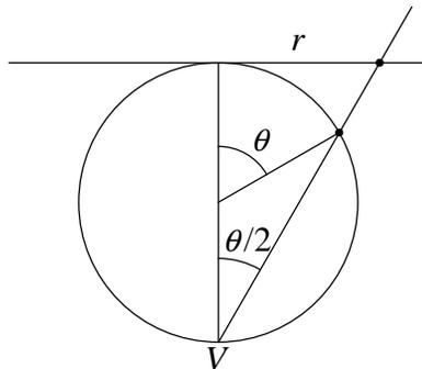
Figure 4. Construction of stereographic projection.
