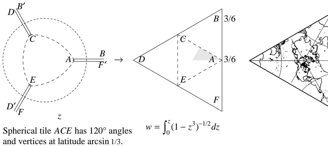
Spherical tile ACE has  $120^\circ$  angles and vertices at latitude  $\arcsin 1/3$ .
