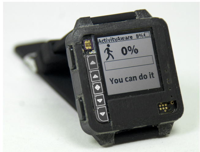
Figure 1: Amulet wrist-worn mHealth platform
