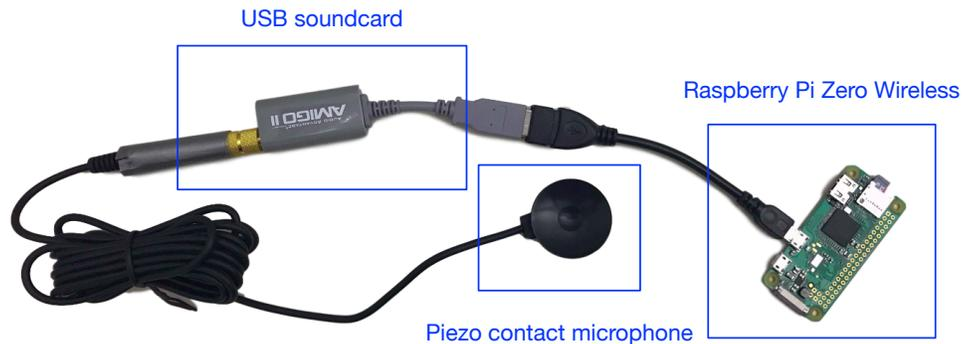
Fig. 5. Raspberry Pi Zero W, external USB soundcard, and piezo microphone. An amplifier was only required due to a software driver issue and hence was left out of the picture. The photo only shows one microphone but our experimental apparatus included four similar microphones connected through a USB hub.
