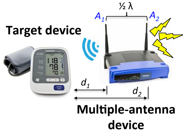
Figure 1: A multiple-antenna device uses antenna A_1 to send a data signal to a target device located at distance d_1 , while antenna A_2 located d_2 from the target transmits barrage jamming (random noise).
