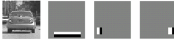
Figure 5: Haar-like features used for car detection (figure source: [4])
