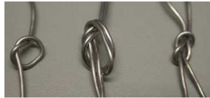
(c) Knots tied by manually using the knot boxes (overhand, double overhand, square)
