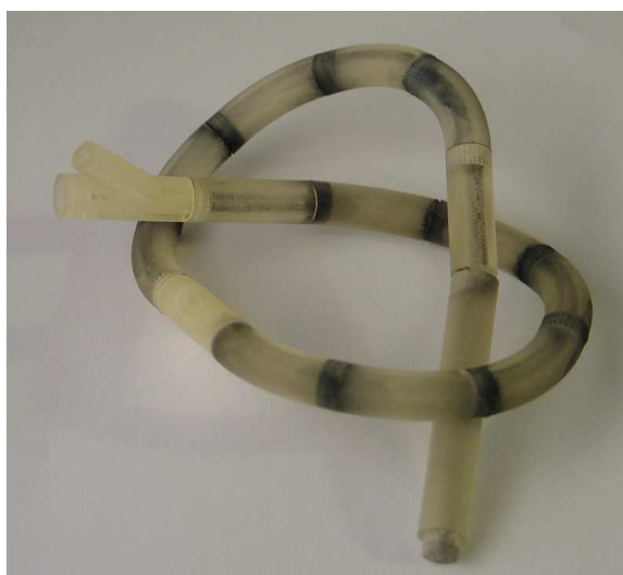
Figure 4.30: Overhand knot formed using the modular components, with two air jet segments (the two lighter colored segments)
