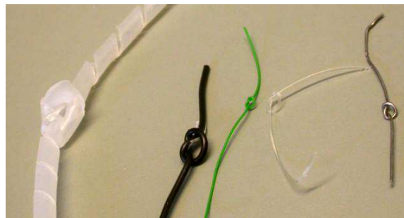
Figure 4.22: Overhand knots in different materials tied manually using the knot box (R to L: .032" solder, fishing line, 30 and 22 AWG wire, wire loom)
