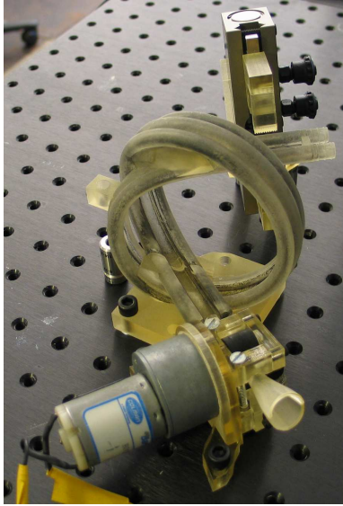
Figure 1.3: Track-based fixture for an overhand knot
