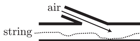
Figure 4.5: Single air nozzle in tube
