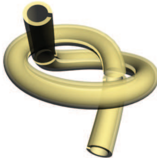
(c) Knot tube with cuts to make extraction easier
