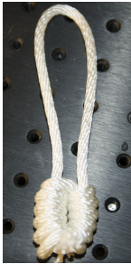
Fig. 13: Non-planar knots, such as those shown here, cannot be tightened using our fixtures.
