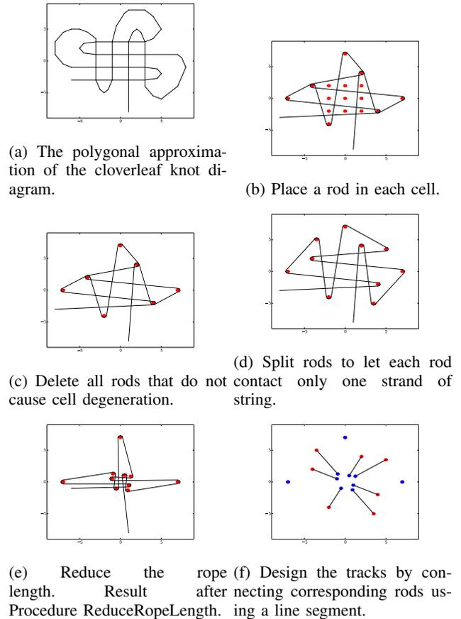
Fig. 7: Automated design of the fixture for the cloverleaf knot using Procedures RodPlacement to ReduceRopeLength.
