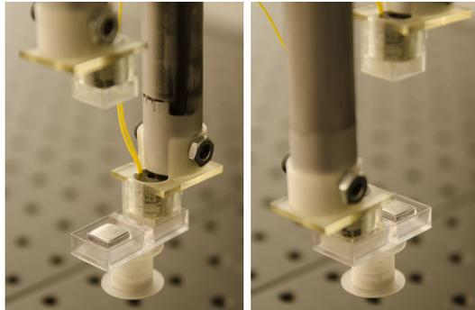
Fig. 4: Two different configurations of the gripper grasping the spool used to arrange the knots.
