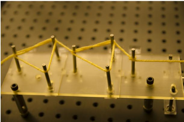
Fig. 10: The first knot unit along the sounding line is tightened around the stationary pin.
