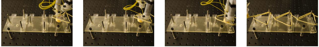
(a) Before re-grasp task in the first unit. (b) After the re-grasp task in the first unit. (c) About to finish arranging for the first unit. (d) Finished arranging three units of sounding line.
