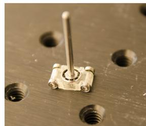
Fig. 5: The slider used for moving rods. The base has four wheels that are made of small ball bearings, while the rod is also on a ball bearing.
