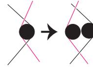
Fig. 6: When multiple strands of string contact the same rod, double the rod.
