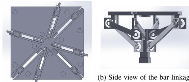
(a) Top view of tracks for a link lengths, to move different cloverleaf knot. (b) Side view of the bar-linkage system. There are two different link lengths, to move different rods with different speeds.
