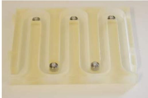
**Figure 4.6:** The modular test structure with rollers (silver ball bearings) installed at every turn.
