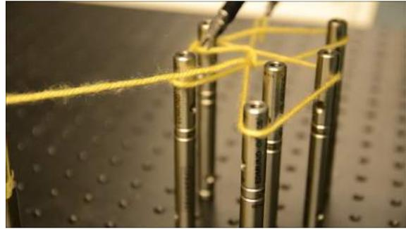
(b) Completing the arrangement of a double coin knot with a single re-grasp.
