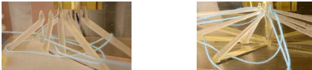
**(a)** Tightening a shoelace unknot, where the knot does not remain flat. **(b)** Tightening a double coin knot, where the knot is not taut.
