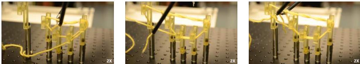
**Figure 5.15:** Arranging a surgeon's knot using a Da Vinci robot arm, around generalized fixtures.
