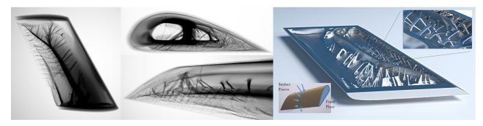
**Fig. 15.** An optimized interior supporting structure of part of a wing is generated using our algorithm on a  $1696 \times 342 \times 1971$  grid (402 M active voxels).
