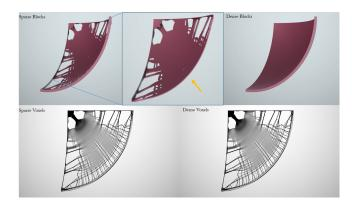
**Fig. 11.** Comparison of the active blocks (top) and the optimized voxels (bottom) using the narrow-band scheme and the dense scheme. We observe negligible difference between the two optimized structures optimized by the narrow-band and dense-grid schemes.
