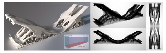
**Fig. 3.** An optimized bridge structure is obtained on a  $271 \times 540 \times 1081$  grid (157 M voxels) with mirror boundary conditions applied on the X and Z axes. The left figure shows a solid render, and the right three figures show the visualization of the density field from different camera views. The middle sub-image illustrates the boundary conditions, including fixed boundaries on the sides and a load applied on the bottom plane.
