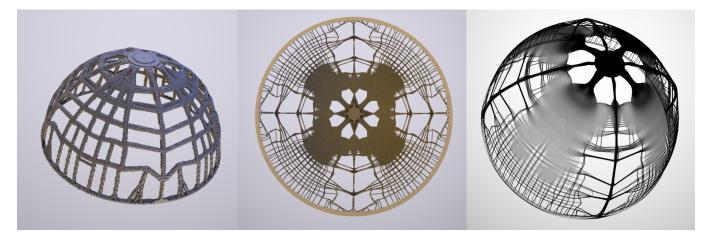
**Fig. 2.** Structures with codimensional thin features are obtained by running the narrow-band algorithm on a thin hemispherical shell. The boundary conditions include a fixed boundary on the top and an external load applied on the cross surface on the bottom. As the grid resolution increases from to 512<sup>3</sup> (left) to 2048<sup>3</sup> (right), thin-shell structures are observed to dominate, matching the tendency studied in [Sigmund et al. 2016].
