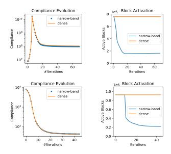
**Fig. 10.** Comparison of the compliance evolution (left column) and the number of active blocks (right column) for the narrow-band and the standard dense topology optimization algorithms on the bridge (top row) and the hemispherical thin shell (bottom row). Note that the increase of the compliance in the first few iterations of the bridge example is due to progressively decreasing volume fraction to accelerate convergence.
