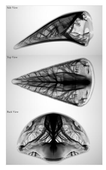
**Fig. 1.** The interior structures supporting the shell of a bird beak generated using our narrow-band topology optimization algorithm with  $k_1$ , 040, 875, 347 (1.04 billion) active FEM voxels. The resolution of the background grid is  $3000 \times 2400 \times 1600$ . The three figures show the volumetric rendering of the same structure from different views.
