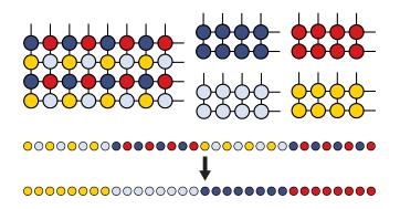
**Fig. 6.** Left: a SPGrid block of 4x8 in which the nodes are ordered lexicographically, Right: the transposed colored storage enables efficient vectorization for Gauss-Seidel iteration. Bottom: Transposition operation of a SPGrid block illustrated in a linear memory layout.
