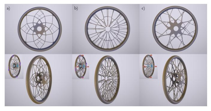
Fig. 14. Optimized wheel structures are generated using our algorithm. Structure (a) and (b) are obtained with in-plane tangential force boundary and out-of-plane normal force boundary. Structure (c) is optimized with a linear combination of objectives in both (a) and (b).
