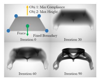
**Fig. 8.** Unbounded topology optimization for a quadpod structure. A thin membrane is initialized (a), evolved upwards (b), and converge to a clear structure (c and d), guided by a combined objective of both minimum compliance and maximum height.
