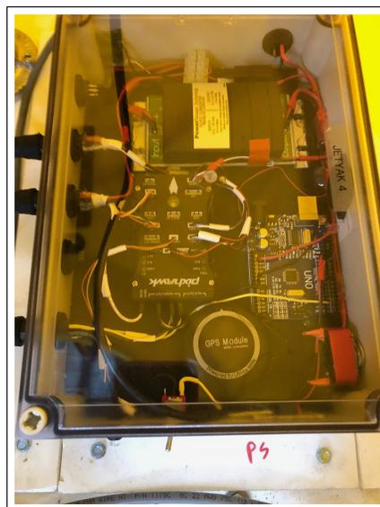
Fig. 5. Electronics box of the ASV, which contains controllers and sensors, including GPS and Arduino. Each of the components can be a source of noise.
