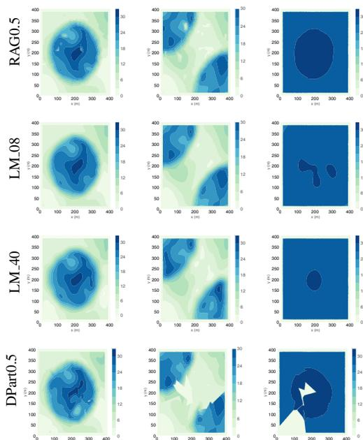
Fig. 4. Sample reconstruction of spatial fields using 6 robots – *SF1* (left), *SF2* (Center), *SF3* (Right) – while the methods indicated at each row. *RAG* accurately reconstructs all the spatial fields, while *DPart* leaves some gaps. Lawn mower generally is able to reconstruct the spatial fields with some inaccuracies dependent on the interlap spacing.
