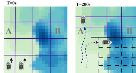
Fig. 1. Sample scenario of the problem considered in the paper: Given an unknown non-stationary field with unique regions, A and B, and multiple robots that are tasked to collect data to reconstruct the spatial field. Is it possible to adapt the sampling path to ensure a certain predictive accuracy (e.g., left vs. right grid) and at the same time minimize the task cost?
