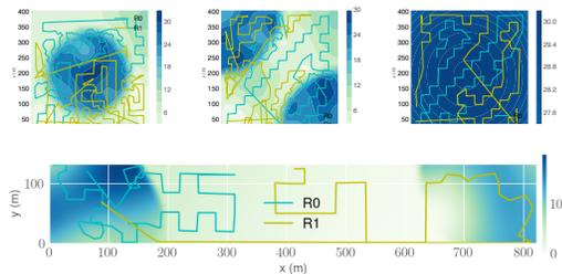
Fig. 5. Trajectories with *RAG* of a 2 robot team after the mission in *SF1* (Top Left), *SF2* (Top Center), *SF3* (Top Right) and *SF4* (Bottom) environments. Robots sample more densely at the *boundary* of the two homogeneous regions than in the homogeneous areas. This demonstrates the robustness of our method in sampling non-stationary fields.
