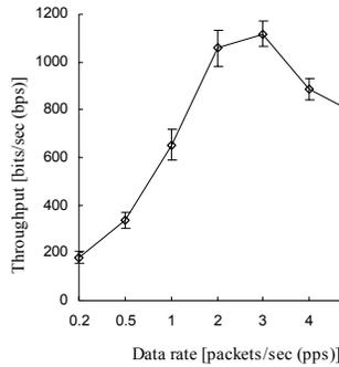
Figure 2. Throughput of CSMA with varying data rates
