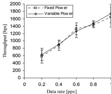
Figure 8. Throughput with fixed/variable beacon transmission power
