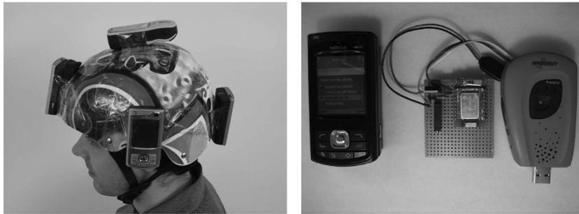
(e) Ground-truth video/sound/photo helmet with (f) BikeNet mobile SAP implementation. The four N80s and GPS receiver, only for use in de-Nokia N80 Bluetooth radio associates with a bugging our system and validating our inference custom-built Bluetooth/802.15.4 gateway techniques.
