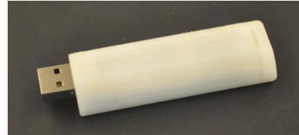
Figure 8. Our Custom Field-Ready Casing on an Atmel RZUSBSTICK
