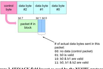
Figure 3. SEQ/ACK field layout as used by the NUSHU protocol.
