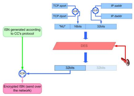
Figure 7. The encryption algorithm for ISN numbers.
