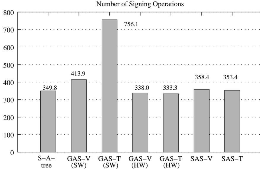
**Figure 7.3:** Counts for signing operations. Numbers for S-BGP, S-BGP(cp), SAS, and SAS with caching are 22,072, 11,521, 22,303, and 12,035 respectively. They are too large to be shown in this figure.
