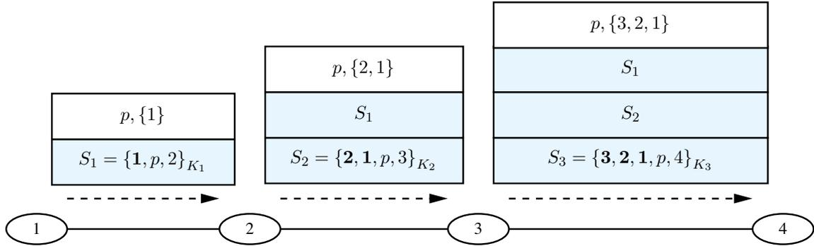
**Figure 4.3:** This figure sketches the process of sending route announcements and their route attestations. We have four ASes numbered as 1, 2, 3, and 4. The figure shows the AS path components in bold.
