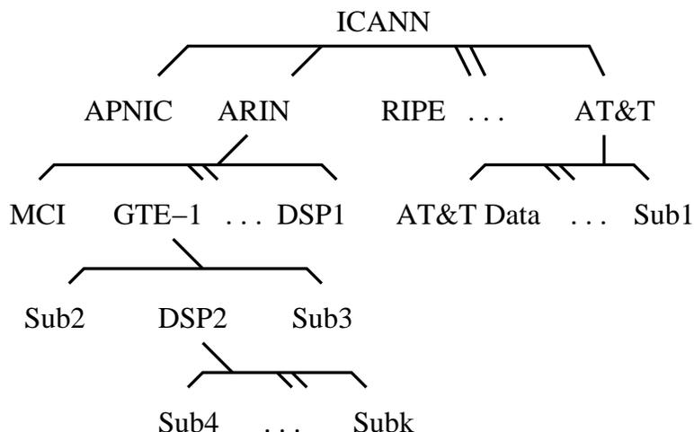
**Figure 4.1:** Sketch of the S-BGP PKI for IP address allocation. The root of the hierarchy is ICANN [80]. The next tier are the large organizations to whom ICANN assigns a large portion of IP addresses. Subsets of their IP addresses are further assigned to smaller organizations.
