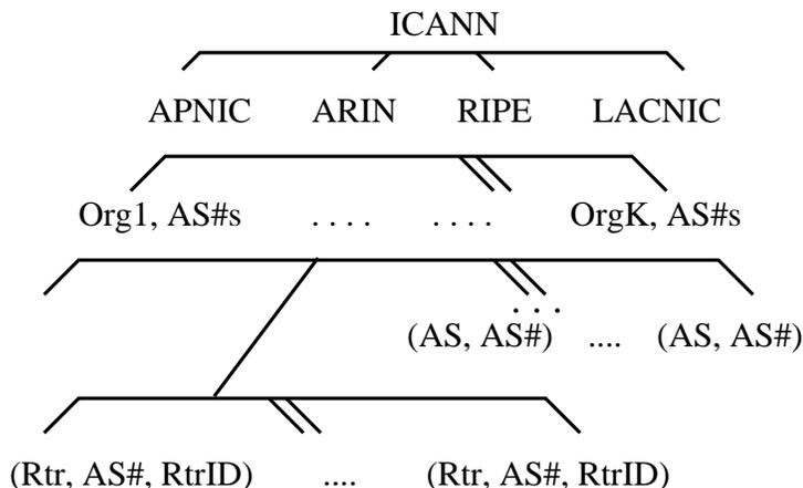
**Figure 4.2:** Sketch of the S-BGP PKI for AS numbers and routers. A certificate for AS number binds an AS with its public key and AS number. A certificate for router binds the router ID with the router’s public key and the AS that the router is authorized to speak for.
