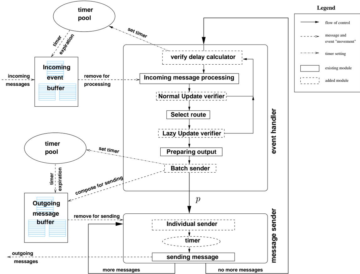
**Figure 3.1:** Simplified flow control model for BGP Update processing with a security system. In a simulation, processing delay  $p$  is imposed after an event is handled, but before outgoing messages are sent. We borrow the diagram of the facility structure from [138] and illustrate our additions using the dash-bordered boxes.
