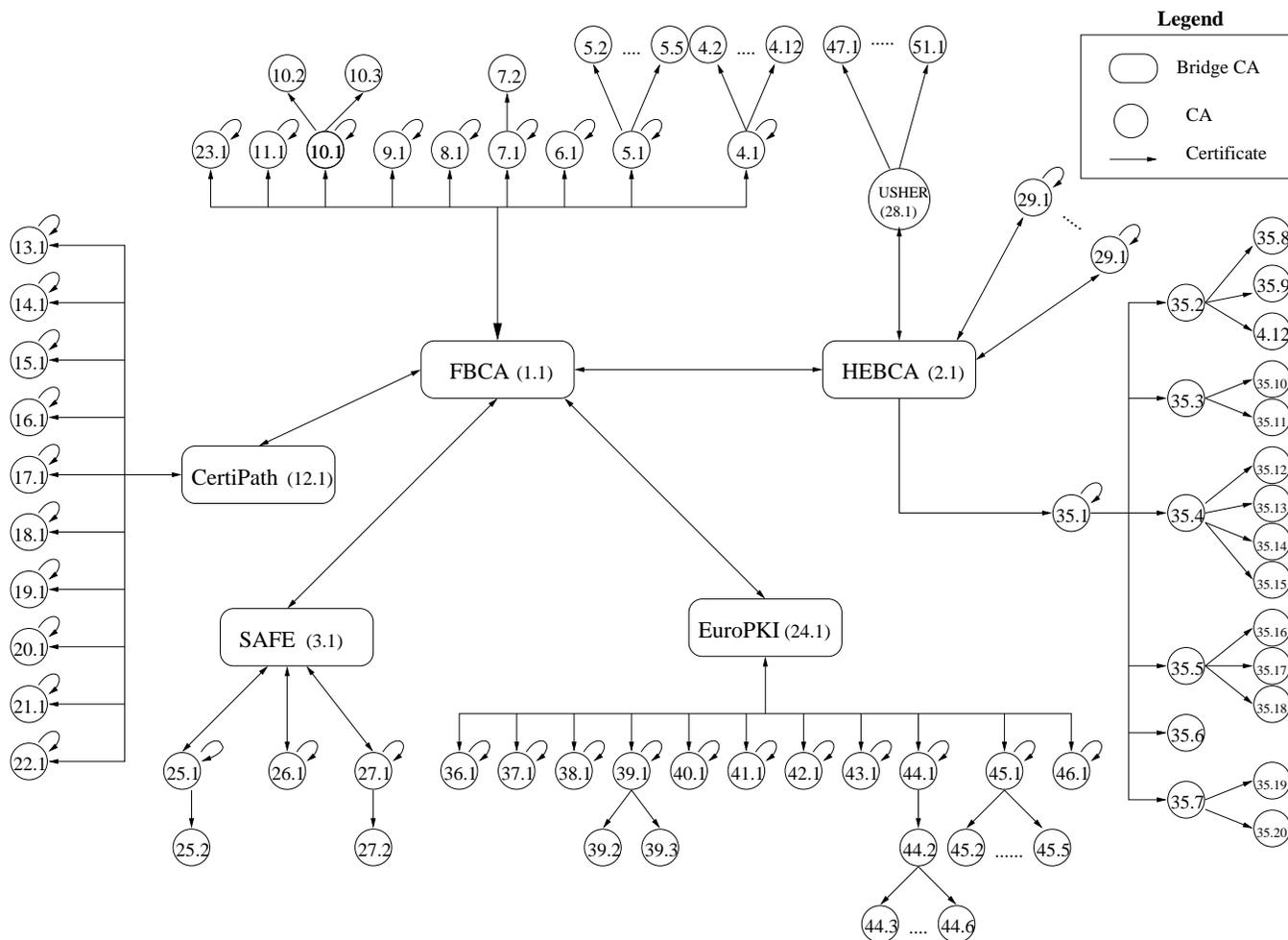
**Figure 10.4:** The configured certificate topology for experiments. The topology is a combination of current deployment and future plans. Each CA with a self-issued certificate can be treated as a trust anchor. The unique ID for each CA is the tuple: (domainID, caID). We assign an index number to each CA in the model for simple implementation.
