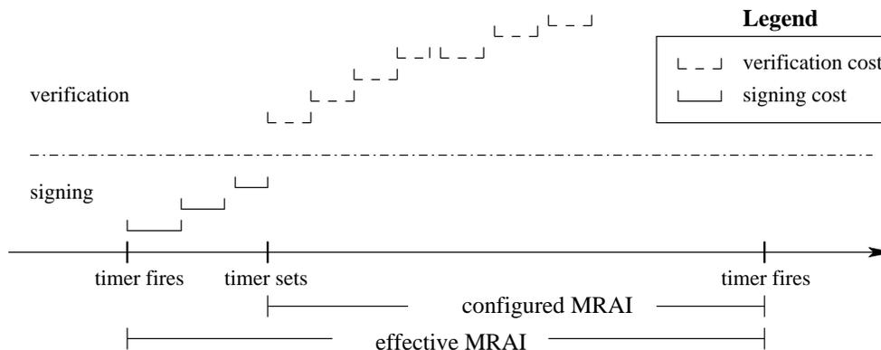
**Figure 6.6:** An example of how the timing of signing and verification operations affect the MRAI timer. Signing latencies associated with message sending effectively prolong the actual MRAI timer value.
