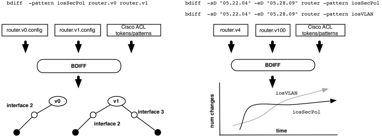
Figure 4: Using *bdiff*, a network administrator may track differences in the implementation of security policy across multiple versions of the same router. Here, the administrator may either specify two versions of the same router to compare or sequentially compare versions of the router across time via longitudinal diff mode.
