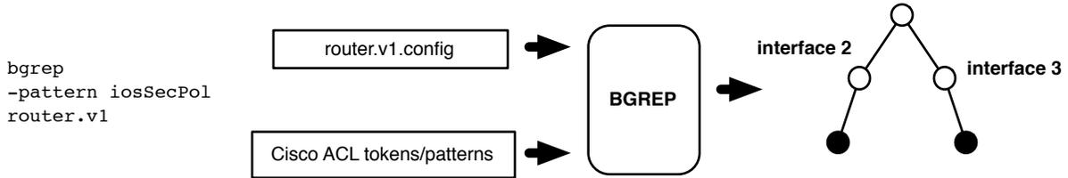
Figure 3: Using *bgrep*, a network administrator may extract blocks of Cisco IOS related to “security policy” within a given router (router.v1). Here, the administrator finds instances of the `service-policy` command within two of the router’s interfaces. Our tool relies upon libraries of lightweight grammars defined for configuration languages, and outputs configuration blocks as parse trees.
