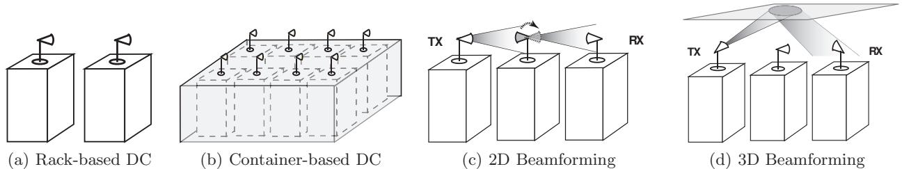
**Figure 1:** Radio transceivers are placed atop each rack (a) or container (b). Using 2D beamforming (c), transceivers communicate with neighboring racks directly, but forward traffic in multiple hops to non-neighboring racks. Using 3D beamforming (d), the ceiling reflects the signals from each sender to its desired receiver, avoiding multi-hop relays.
