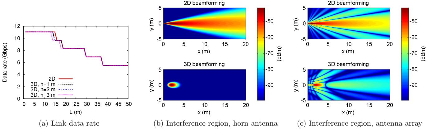
**Figure 2:** Key properties of 3D Beamforming. (a) Data rate vs link distance  $L$ . (b)-(c) 2D and 3D beamforming signal maps using both horn antenna and antenna arrays. The transmitter is at (0m,0m) and the receiver is at (2m,0m).
